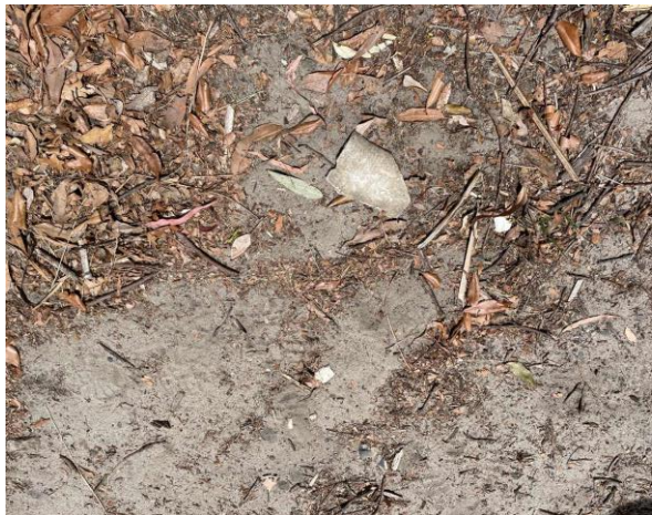
Line ID 13: External, Rotunda Canopy, Ground Floor, Debris to Soil Adjacent Rotunda Canopy, Moulded Fibre Cement Debris - Chrysotile Asbestos Detected
