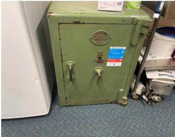
Line ID 25: Internal, Office Building, Ground Floor, First Aid Room, Rope Insulation to Safe, Woven Material - Suspected Asbestos
