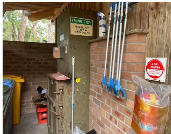
Line ID 34: External, Office Building, Ground Floor, Baler, Green Paint - Lead Detected (0.46% w/w)
