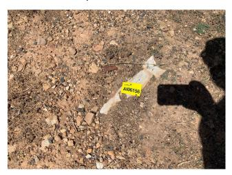
Line ID 13: External, Grounds South Adj to Yarraman/Meroo Lodges, East Adj to Visiting Staff Lodges, Protruding Redundant Pipe, Moulded Fibre Cement - Chrysotile and Amosite Asbestos Detected
