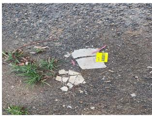
Line ID 99: Internal, Maintenance Workshop, Elevations, East Adjacent to North Portion of East Wall, Ground Surface, Debris, Compressed Cement Sheet Debris - No Asbestos Detected
