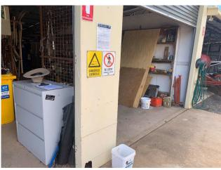
Line ID 27.1: External, Maintenance Workshop, Elevations, Workshop South & North Wall & Machinery Shed North, Wall Cladding and Joinery, Compressed Cement Sheet - Chrysotile & Amosite Asbestos Detected
