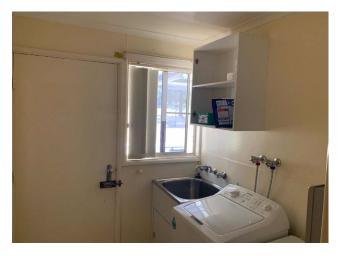
Line ID 78: Internal, General Managers Residence, Laundry, Wall Lining, Compressed Cement Sheet - Chrysotile Asbestos Detected
