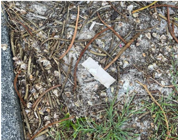
Line ID 12: External, Murphy's Cottage Block, Veranda and Undercover Area, Debris to the Floor From the Eave to Rear of Kitchen, Fibre Cement Debris - Chrysotile Asbestos Detected
